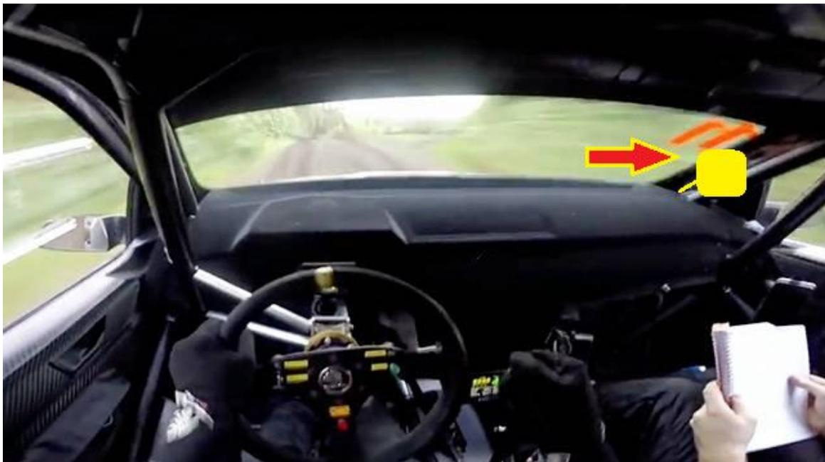
The GPS should be placed on the right pillar of the front part of the safety cage.
